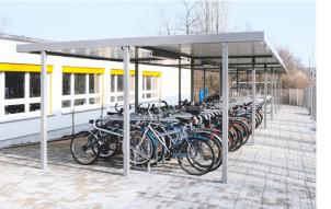
Roofed bicycle stands that enable the user to lock the front wheel to the bicycle stand are ideal. Avoid solutions that only stabilise the front wheel.
